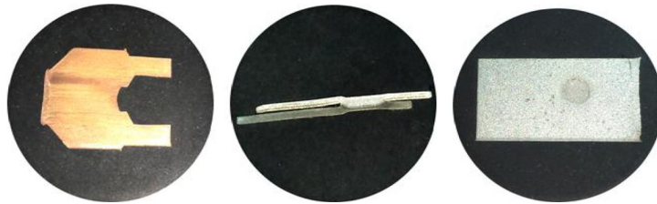
Figure 2. Hot press mounted samples for SEM scanning.
