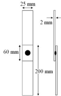
Fig. 1. Welding Sample with Dimension.
