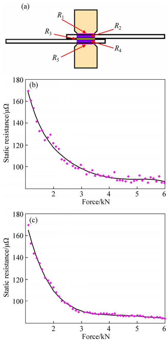
**Fig. 3** Various resistive components in static resistance (a) and static resistance of pneumatic based system (b) and static resistance of servo based system (c)
