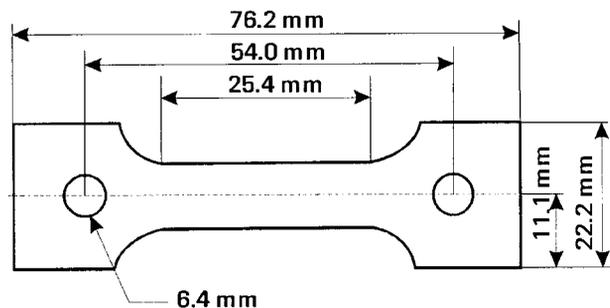
7 Schematic diagram of tensile specimen
