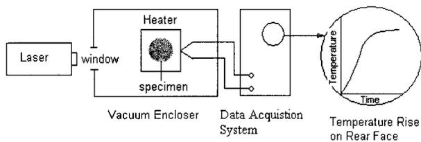
4 Schematic diagram of laser flash apparatus for measuring thermal diffusivity of material
