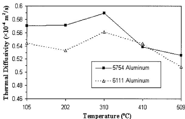
5 Thermal diffusivity of 5754 and 6111 aluminium alloys
