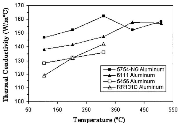
6 Thermal conductivity of 5754 and 6111 aluminium alloys, as well as 5456 and RR131D aluminium alloys
