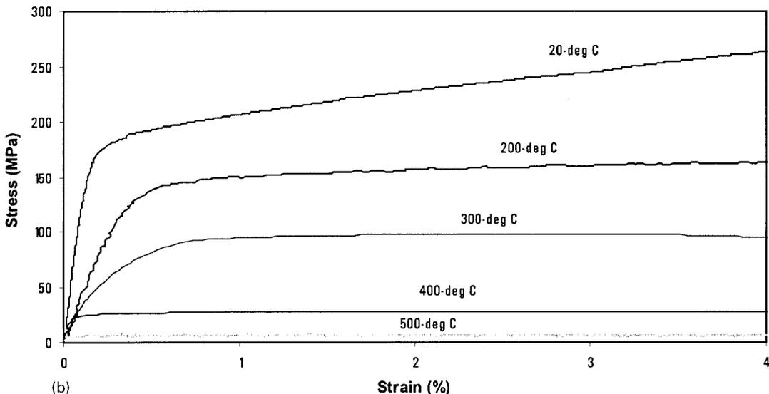
9 Typical tensile stress-strain curves of a 5754 and b 6111 aluminium alloys as a function of temperature
