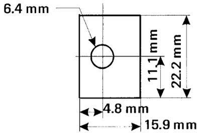
8 Schematic diagram of tab welded to end of tensile specimen
