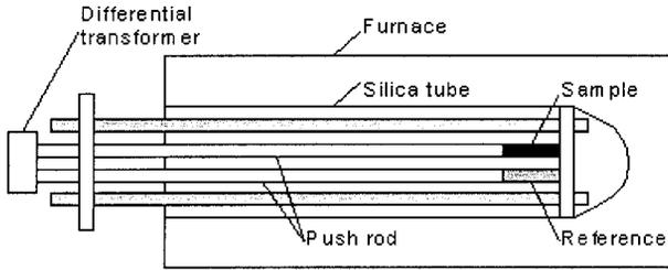
1 Schematic diagram of differential dilatometer
