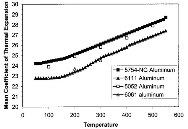
2 Mean coefficient of thermal expansion of 5754 and 6111 aluminium alloys, as well as 5052 and 6061 aluminium alloys
