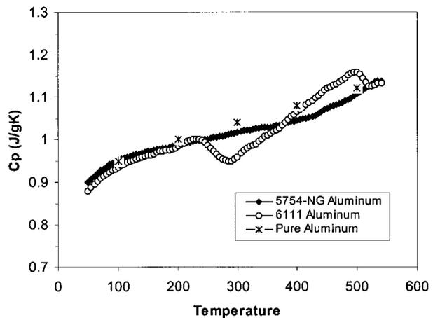
3 Specific heat of 5754 and 6111 aluminium alloys, as well as pure aluminium
